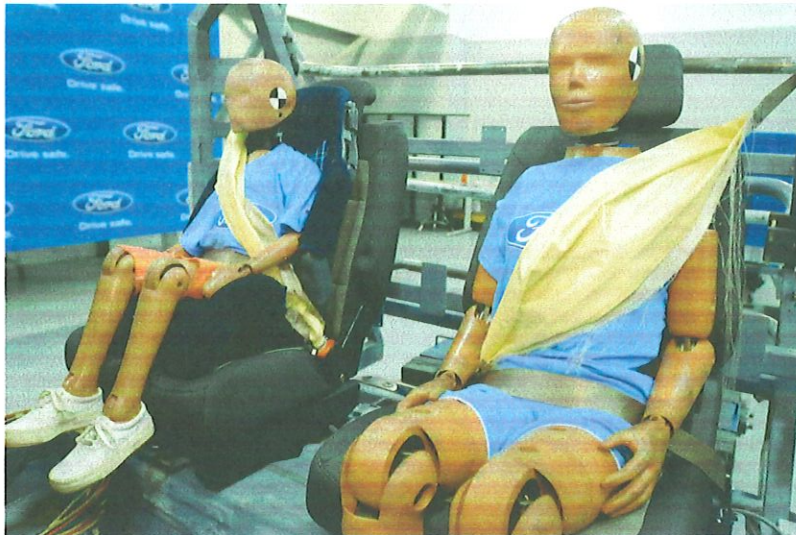
A seatbelt that inflates like an airbag, spreading the force over a wider area, was introduced as an option on the 2011 Ford Explorer. Ford Motor
